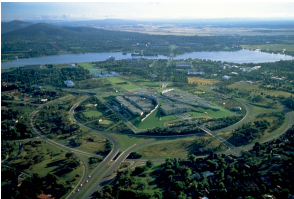
Photograph of Australia's Parliament House from the air. The two curved walls separate the two chambers. The public entrance is closest to the lake and opposite that entrance is the ministerial wing.
