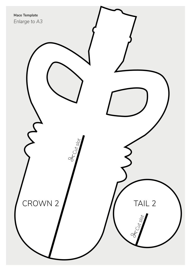
c) Cut the crown and tail pieces. Make sure that the width of each slot in the crown and tail pieces is equal to the thickness of the MDF, plywood or cardboard that you are using.
